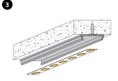
Secure extrusion to surface.
