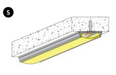
Snap lens onto extrusion.
