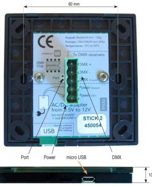
**PORT**: Scratch away sticker over 2 dots shown. Solder wires to the exposed solder points. Connect these to trigger a single scene to start
