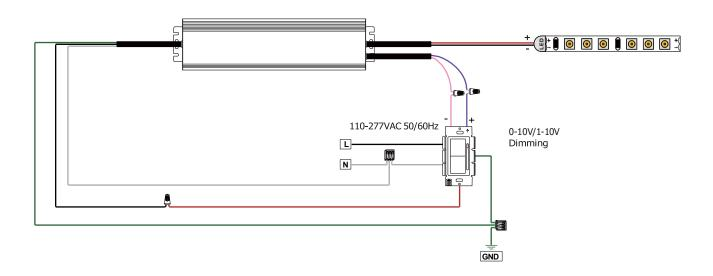
D.0-10V/1-10V Dimmer Wiring Diagram (The driver is independently connected to the input.)
